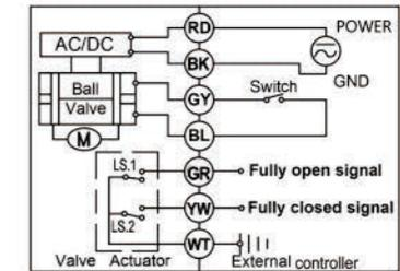
■ CR701 Wiring Diagram (7 wires control with feedback signal)
