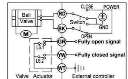
■ CR502 Wiring Diagram (5 wires control - Capacitors return in case of the power is failure & feedback signal)
