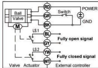
■ CR705 Wiring Diagram (7 wires control - Capacitors return in case of the power is failure & feedback signal)
