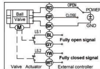
■ CR706 Wiring Diagram (7 wires control - Capacitors return in case of the power is failure & feedback signal)
