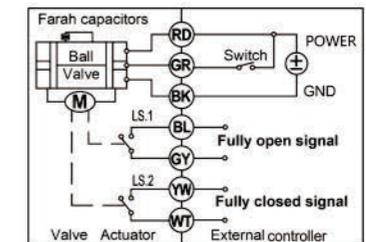
■ CR703 Wiring Diagram (7 wires control with feedback signal)
